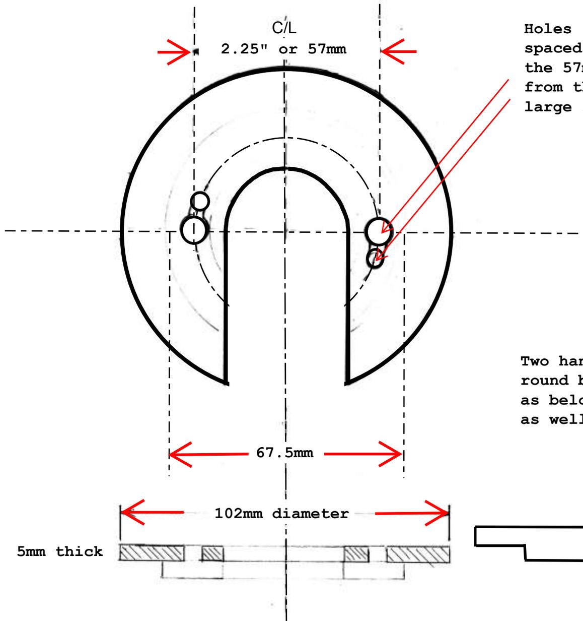
Holes 10.5mm and 6.5mm spaced 11mm apart around the 57mm circle slotted from the smaller to the large following the circle.
